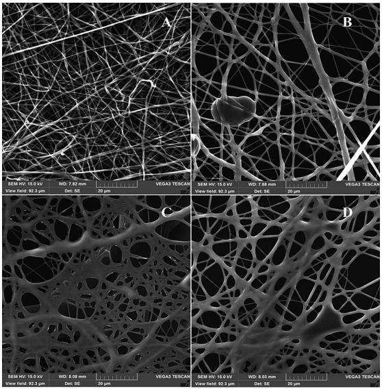
**Figure 2.** Electron microscopy image of the PVA Povidone-iodine functionalized nanofibers A) PVA Povidone-iodine functionalized nanofibers at the beginning of the test,
