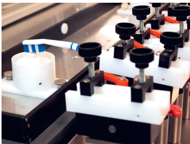
Obr. 3 Simulátor zubního kartáčku - toothbrushing machine [http://sdm-gmbh.de/en/products/toothbrush-simulation-zm-38-and-zm-312.html]
