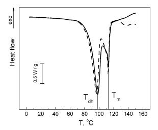
Fig. 8. Normalized DSC thermograms of MgSt (solid line) and MgSt: MgLac (dashed line). The vertical lines indicate the dehydration temperature  $(T_{\it dh})$  and the melting temperature  $(T_{\it mr})$  of MgSt.
