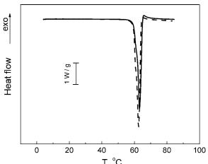
T, °C Fig. 7. Normalized DSC thermogram of TA melting: individual TA (solid line); mixture TA: MgLac 1: 4 (w/w) (dashed line)
