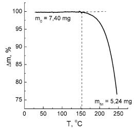
Fig. 5. TGA curve of TA sample. The dotted lines are plotted to show the limit of thermal stability of the TA. The values of initial and final sample mass ( $m_0$  and  $m_{\rm fin}$  respectively) are indicated.
