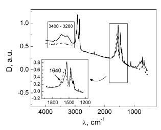
Fig. 4. FTIR spectra of MgSt in the initial state (solid line) and after drying (dashed line)
