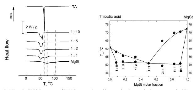
Fig. 2. a) Normalized DSC thermograms of TA-MgSt mixtures (vertical lines are plotted to trace the characteristic peaks of TA and MgSt); b) binary phase diagram of TA-MgSt melting. MgSt: TA molar ratios are indicated beneath the experimental points
