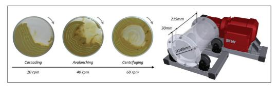
Fig. 1. Left – dynamic behaviour of GoldCell® selenium yeast in the rotating drum with increasing rotation frequency, right – the rotating drum
