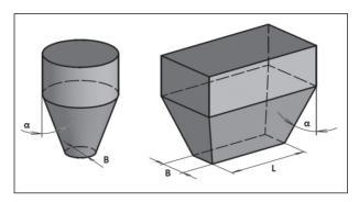
Fig. 3. Schema of the hopper geometry for axially symmetrical (left) and plane flow (right)
