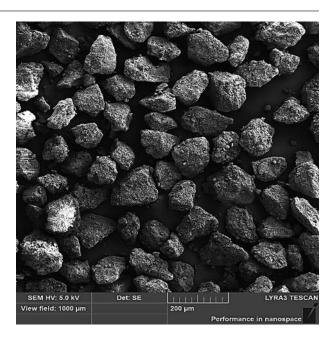
Figure 1. SEM picture of sorbitol particles
