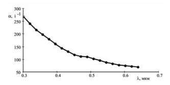
Fig. 1. The attenuation spectrum of the suspension of  ${\rm Ag@Fe_3O_4}$  nanoparticles
