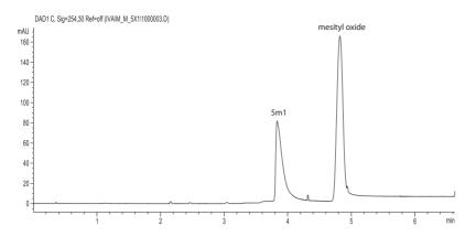
Fig. 1. Electropherogram of compound 5m1 (7.5.10–4 mol.l $^{-1}$ ) and mesityl oxide (2.10–6 mol.l $^{-1}$ ) in MOPSO/NaOH background electrolyte (pH = 6.70, I = 0.01 mol.l $^{-1}$ ), injection by pressure 40 mbar for 4 s, applied voltage +15 kV, temperature 25 °C, detection at 254 nm
