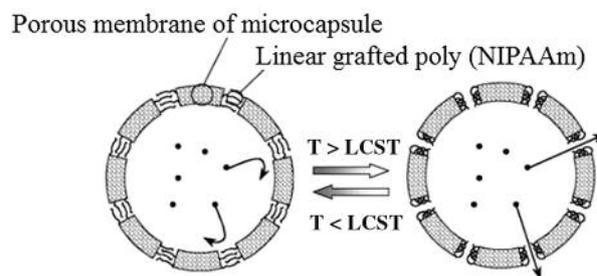
Fig. 8. The thermo-responsive release principle of the microcapsules with a porous membrane and the TR polymeric gates (modified from<sup>28</sup>)
