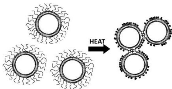
Fig. 7. The scheme of the thermo-responsive behaviour of the liposomes modified with the TR polymers<sup>46</sup>
