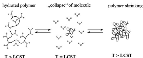
Fig. 4. The thermo-sensitive behaviour of the TR polymer pNIPAAm (modified from<sup>24</sup>)
