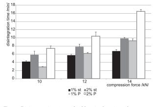
Fig. 3. Disintegration time of tablets in function of compression force – Disintequik<sup>TM</sup> MCC with lubricants st – magnesium stearate, P – poloxamer 407
