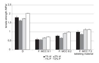
Fig. 2. Tensile strength of tablets at the compression force of 14 kN D – Disintequik<sup>TM</sup> MCC, F – Flowlac® 100, MCC – Microcel® MC-102, st – magnesium stearate, P – poloxamer 407
