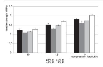
Fig. 1. Tensile strength of tablets in function of compression force – Disintequik  $^{\text{TM}}$  MCC with lubricants st – magnesium stearate, P – poloxamer 407
