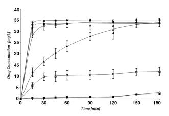
Fig. 5. The dissolution behaviour of diclofenac sodium (100% ~ 35 mg) in dissolution media of different pH values: ♦ phosphate buffer pH 2.0; ■ McIlvaine's buffer pH 3.2; □ phosphate buffer pH 4.5; ▲ McIlvaine's buffer pH 6.8 △ phosphate buffer pH 7.4; ● phosphate buffer pH 8.0; and ○ purified water Note: drug concentration of 35.0 mg.l-1 ~ 100% drug release
