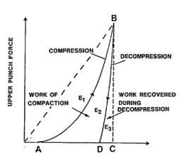
Fig. 1. Plot of upper punch force versus upper punch displacement during compression and decompression  $E_1$ —energy of friction,  $E_2$ —energy accumulated by the tablet, E3-energy of decompression
