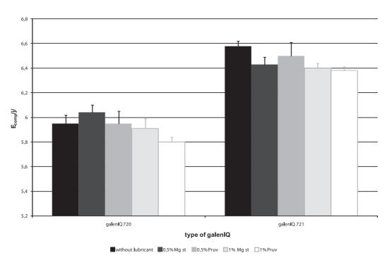
Fig. 5. Values of energy of compaction at the compression force of 8 kN  $E_{\rm comp}$  – energy of compaction, Mg st. – magnesium stearate
