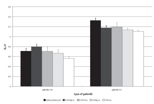
Fig. 3. Values of energy accumulated by the tablet at the compression force of 8 kN  $E_{\rm 2}$  – energy accumulated by the tablet, Mg st. – magnesium stearate
