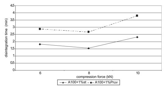
Fig. 4. Disintegration time in function of compression force: Advantose 100 with lubricants
