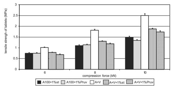
Fig. 3. Comparison of tensile strength of tablets: Advantose 100 and its mixture with Vivapur 102 without and with lubricants
