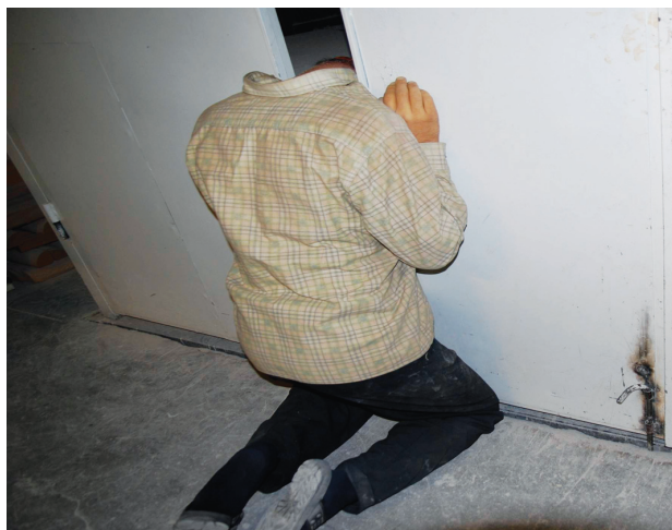
Figure 1. Head and neck lodged within openings of the elevator.
