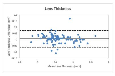
Graph 4. Bland-Altman plot for the lens thickness measurements of each device
