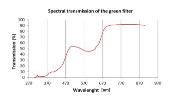
Fig. 1: Spectral characteristics of green chromagen filter.
