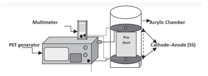
Fig. 2. The PEF generator scheme
