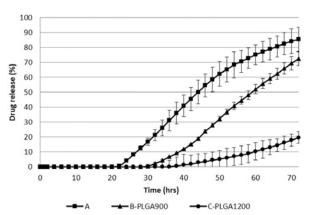
Fig. 3. In vitro dissolution profiles of mirtazapine PLGA microparticles from samples A, B-PLGA900 and C-PLGA1200
