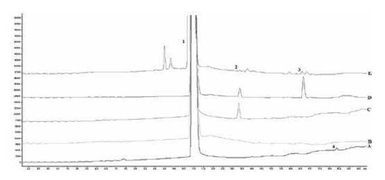
Fig. 3. The chromatogram of degradation studies (A – test, B – acidic, C – temperature, D – alkaline, E – peroxide; 1 – salbutamol sulfate, 2 – impurity D, 3 – impurity G, 4 – impurity F)
