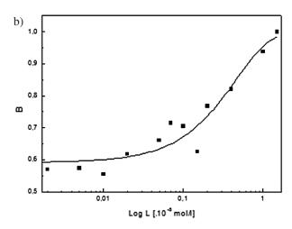
Fig. 2. Langmuir isotherm of HYP/DNA complex (a). L represents the concentration of DNA and B is normalized HYP fluorescence intensity (excitation wavelength: 560 nm). Concentrations are mentioned in the text. Semi-logarithmic representation of binding curve (b). Final binding constant was taken as an average of two ones obtained from a, and b.
