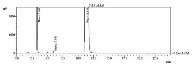
Fig. 1. A typical chromatogram of a pharmaceutical preparation containing sodium picosulfate as the active ingredient, sodium benzoate as the preservative and impurity A, which is the main hydrolytical degradation product of the active substance
