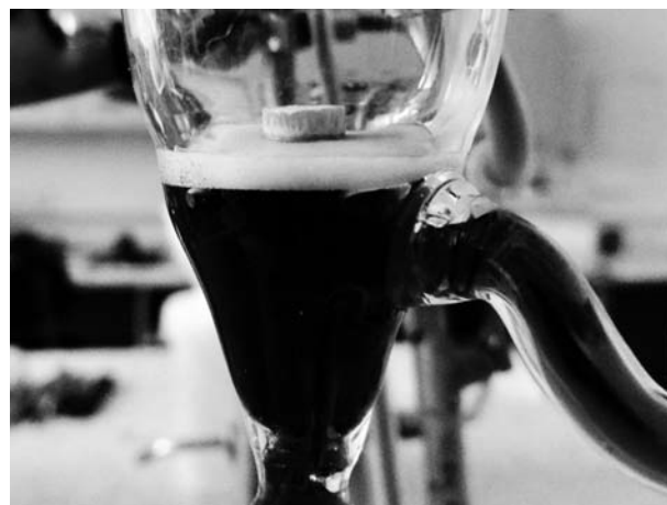
Fig. 1. Water absorption rate test of tablet
