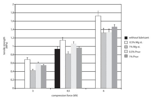
Fig. 2. Tensile strength of tablets in function of compression force: Sorbitab SD 250
