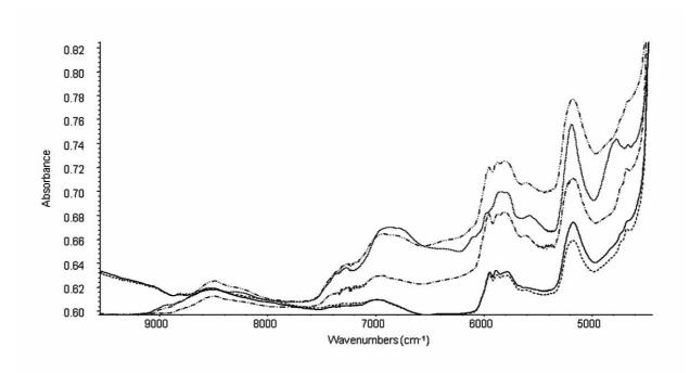
Fig. 1. NIR spectra of separate EL film (-), separate ES film (---), hypromellose hard capsule (...) and capsules coated by EL film (-..-) and ES film (-..-).
