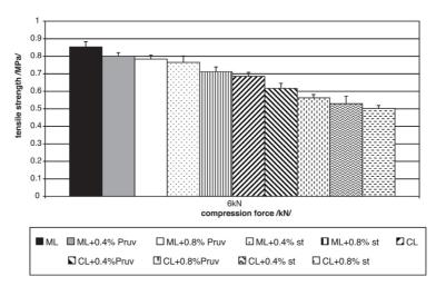
Fig. 3. Tensile strength of tablets - MicroceLac®100 and Cellactose®80 without and with Pruv and magnesii stearas
