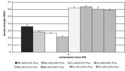
Fig.~6.~Tensile~strength~of~tablets-MicroceLac @100~and~Cellactose @80~with~50%~active~ingredients
