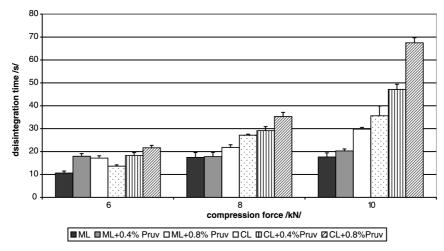
Fig. 2. Disintegration time in function of compression force: MicroceLac®100 and Cellactose®80 without and with Pruv
